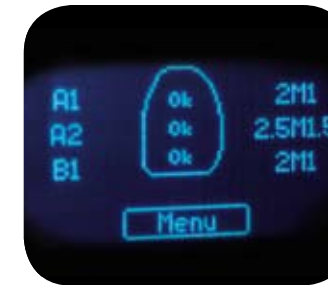
The VITA Easyshade measures a basic overall tooth shade or separates the tooth into cervical, middle and incisal areas, depending on your preference.
