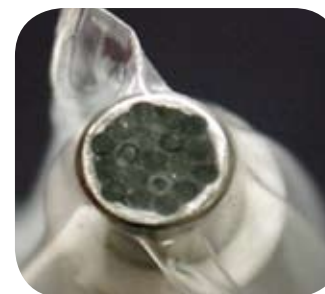
There are 19 individual fiber optics that illuminate the tooth with sensors for the spectrometers to capture every nuance of the shade.
