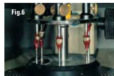
Transfer of the primary parts to the milling platform
